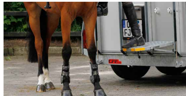
Easy mounting with the climbing aid that can be easily unfolded on the rear ramp; this also puts less strain on the horse's back.
