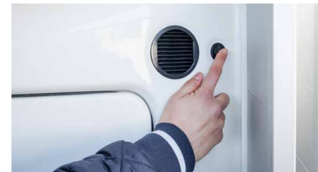
Convenient operation due to the easily accessible and separate light switch for the interior lighting on the right-hand entrance door.
