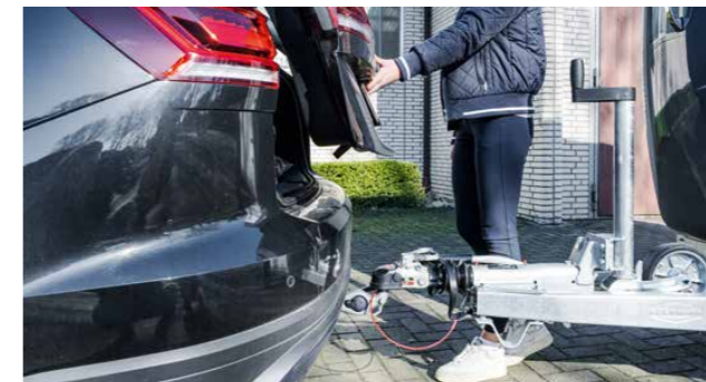
Unimpeded access to the car boot due to the rubberised, convenient heart-shaped coupling handle and the flat brake lever – also when attached.
