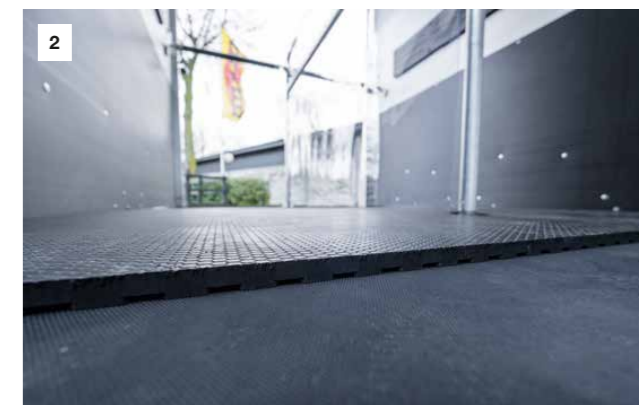
Durability with the kick protection in front of the horses [1] and the wear mat in the area of the front legs [2].
