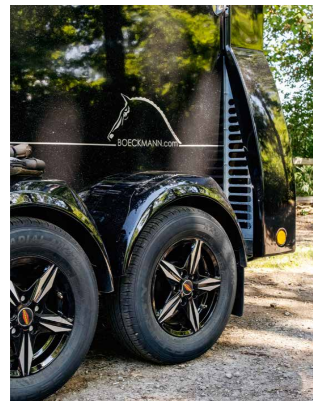
Visual highlight with the polyester cover for side braces, the single polyester fenders, as well as the Böckmann Premium aluminium rims.
