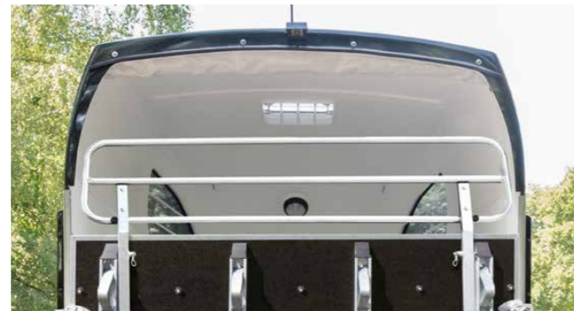
Safety on the road with a folding foal grid.
