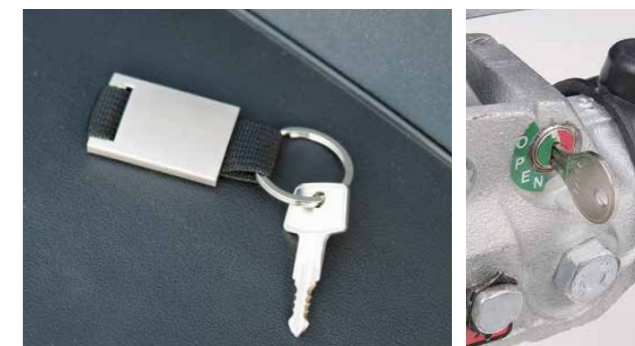
One key for all locks with a master key in triplicate for the tack locker door, access door and cast coupling.
