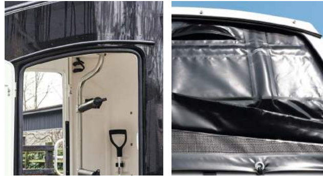
Protection against rain provided by the rain gutters above the doors and also in the rear area.
