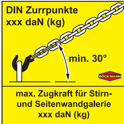
Fig. 5: Lashing points on the trailer
