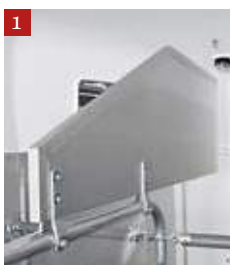
Aluminium head divider wall for transporting two stallions (1) or one head divider wall grating (2) Hodeskillevegg i aluminium for transport av to hingster (1) eller en gitter-skillevegg (2)
