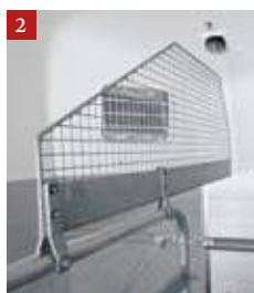
Aluminium head divider wall for transporting two stallions (1) or one head divider wall grating (2) Hodeskillevegg i aluminium for transport av to hingster (1) eller en gitter-skillevegg (2)
