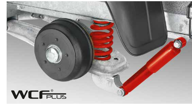
Travelling comfort with the World-Class chassis to automotive standards with wheel shock absorbers.
