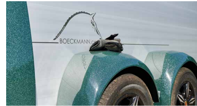
Fenders as shelf with the wide and open, straight form of the impact-resistant plastic or polyester fenders (accessory).
