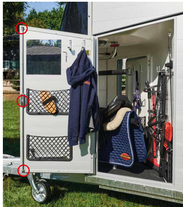
Optimum closure with the 3-point door lock and rubber seal.
