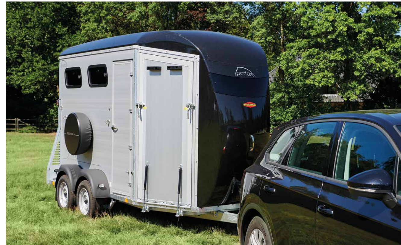
Easy to tow due to the aerodynamic body and low centre of gravity – also saves fuel.
