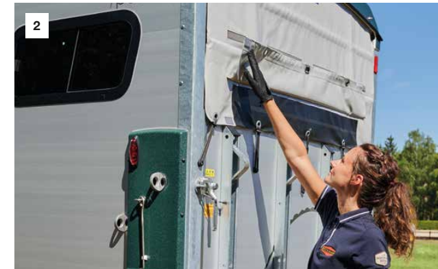
PVC canvas lift with roll-up function [1] and integrated net (not with the Big Portax models) [2].
